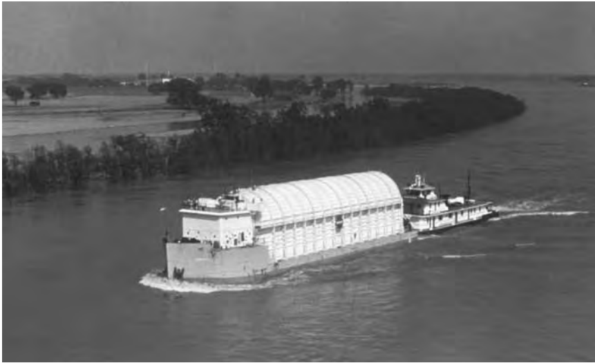
A specially configured barge carries a Saturn booster near the Mississippi test facility.
